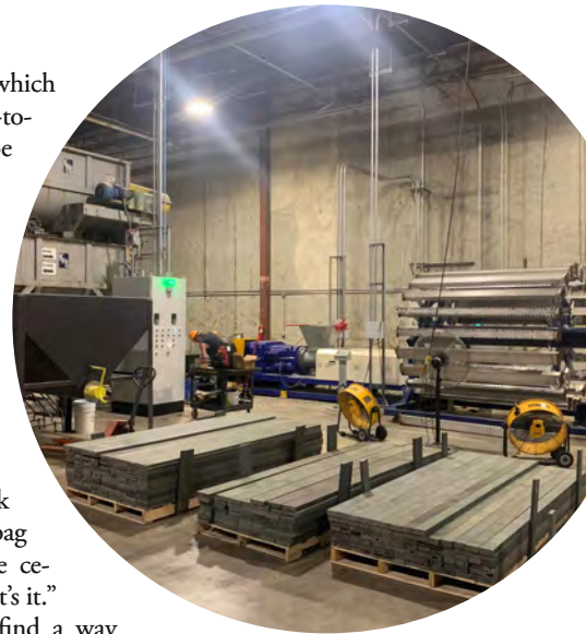
First Star Recycling’s PRF uses plastic lumber manufacturing equipment to create boards in four sizes.
