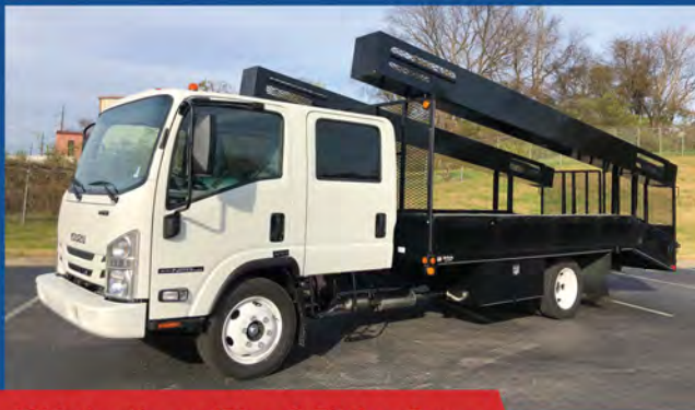
19' Irrigation w/Pipe & Fitting Boxes
