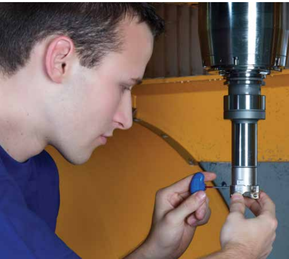
Modular CK precision tool system components use a cylindrical connection with a radial locking screw.
