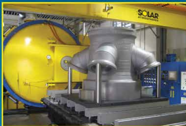
Solar Atmospheres heat treated the titanium manifold weldment used on the Orion Launch Abort System for the NASA Artemis I Program.
