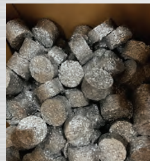
ABOVE: For many aerospace and defense manufacturers, the main motivations to incorporate chip processing and briquetting, such as that from Jorgensen-SFH, are easier chip handling, less chip storage volume and better coolant recovery. LEFT: Loose chips create spatial restraints depending on the shape and size, whereas shops save floor space when forming chips into briquettes with the Jorgensen-SFH system.
