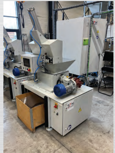
At one aerospace and defense company, its Jorgensen-SFH system accommodates the company's chip bins of all sizes for several machine tools to eliminate the need for forklifts, replacing them with carts that are easily moved to a tipper unit.
