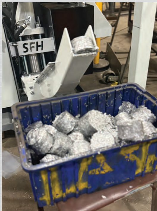
ABOVE: For many aerospace and defense manufacturers, the main motivations to incorporate chip processing and briquetting, such as that from Jorgensen-SFH, are easier chip handling, less chip storage volume and better coolant recovery. LEFT: Loose chips create spatial restraints depending on the shape and size, whereas shops save floor space when forming chips into briquettes with the Jorgensen-SFH system.
