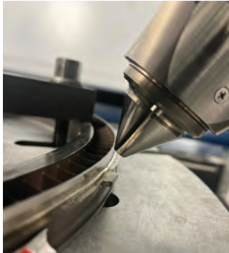
▲ GKN Aerospace DED repair
