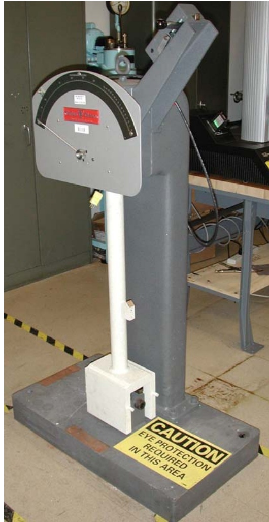
Figure 2.27: Tinius Olsen impact test machine.
