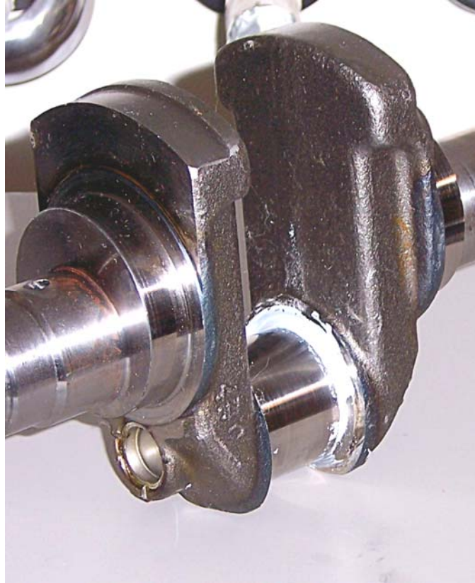
Figure 3.7: Critical fillet area of crankshaft painted to better observe crack.
