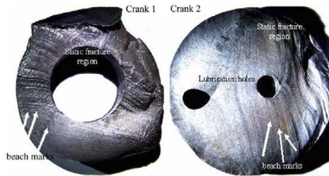
Figure 1.4: Fracture surfaces from failed one-cylinder diesel crankshafts from the study by Bayrakçeken et al. [2006].
