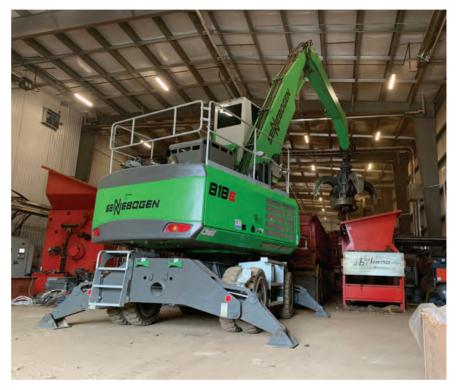
In stationary or mobile applications, rubber-tired material handlers provide excellent agility for operating in confined spaces.
