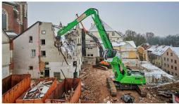
The **SENNEBOGEN 830** tracked demolition machine features a telescoping undercarriage that hydraulically expands from the compact transport mode to wide-stance working platform for stability and safety. Sennebogen offers high-reach capabilities up to 118 feet of reach and a lift capacity of 8,000 pounds fully extended!
