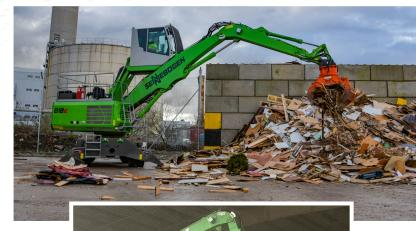
The **SENNEBOGEN 818** making light work of handling C&D materials.
