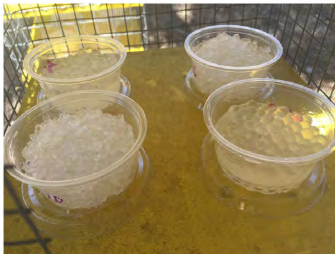
Fig. 23. Gel cups inside of a bait station. From the lower left, clockwise, cups contained PAA, ALG, PAA, and ALG hydrogels. The ALG hydrogels are spherical, and PAA hydrogels have an irregular shape.
