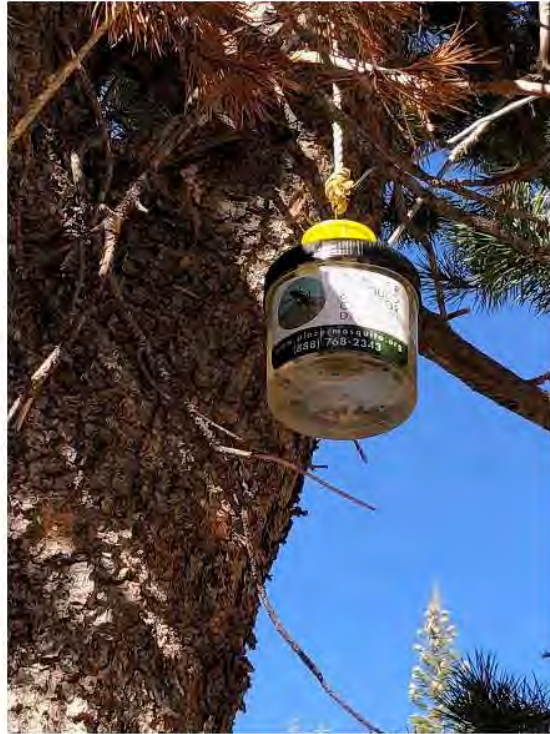
Fig. 1. A Placer-style yellowjacket monitoring trap in the field. These traps were baited with minced canned chicken or heptyl butyrate.
