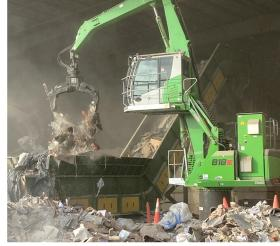
The pedestal-mounted **SENNEBOGEN 818** is a purpose-built C&D and waste handling
