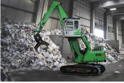
**SENNEBOGEN 818** in tracked and wheeled formats equipped with a two-tine grapple and an orange-peel grapple with 360-degree rotation for maximum control.
