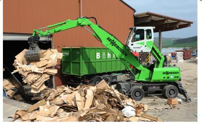
An **818** easily handles plastic bales in the storage area while another feeds an OCC infeed conveyor. The raised cab increases visibility and safety, while its reach allows easy bale stacking and presorting.
