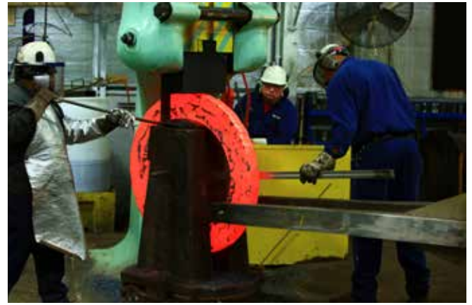
Open die forging can produce custom prototypes faster than any other forging process.
